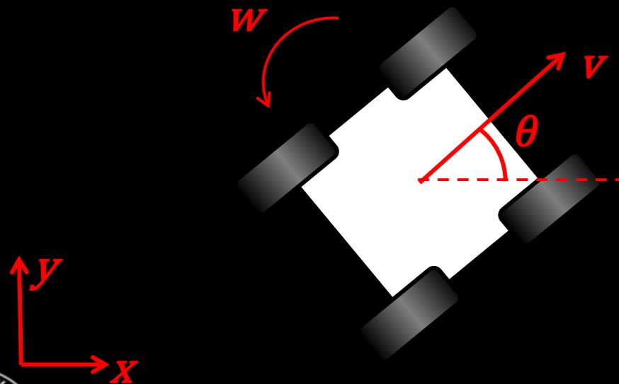
$$\begin{aligned}\dot{x} &= \cos(\theta)v \\ \dot{y} &= \sin(\theta)v \\ \dot{\theta} &= w\end{aligned}$$
