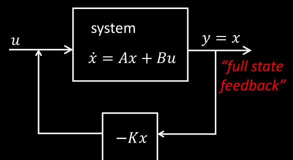
A linear controller (K matrix) can be optimal for linear systems!
