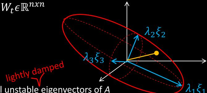
A system is stabilizable iff all unstable eigenvectors of A are in the controllable subspace Fast Robots
